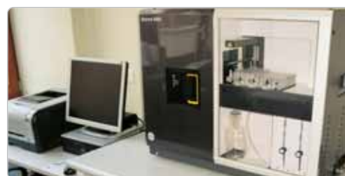
Mass spectrometer with ion trap ESI-HCTUltra, Bruker Daltonics (Transcriptomics and Proteomics Laboratory)
